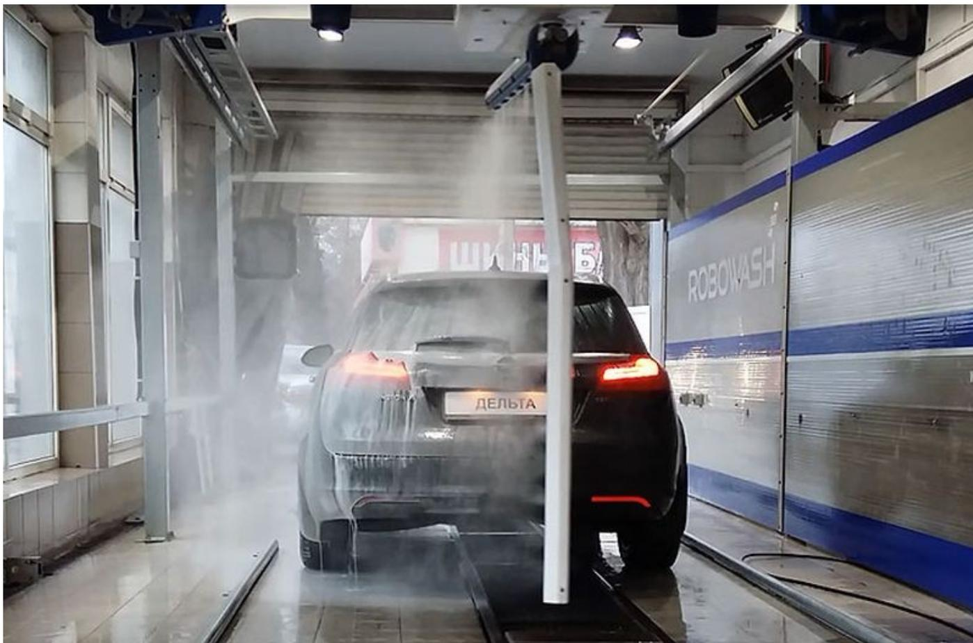
**3. Smart 360 rotate arm, Flush car body 360° with high pressure water.**
